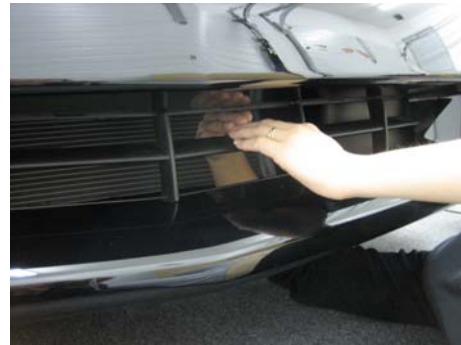
Positioning shown for easy two-handed cable tie installation.
